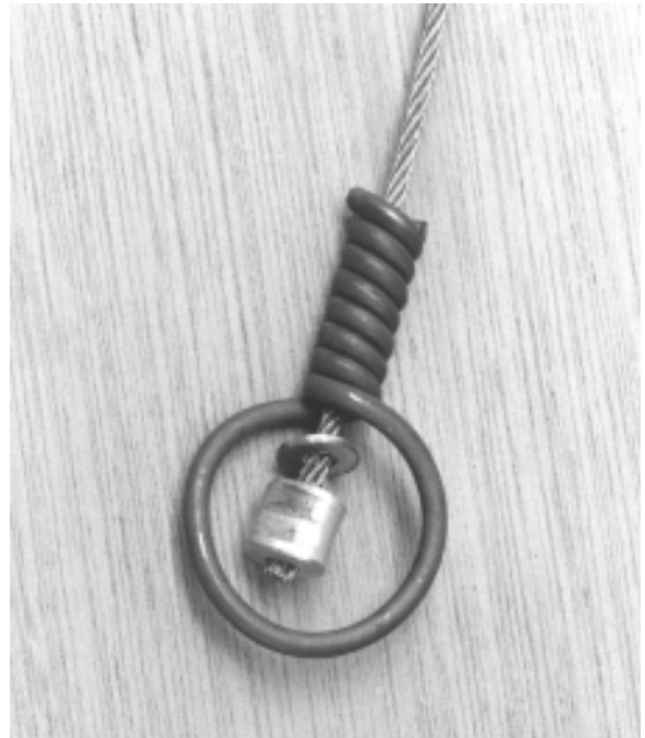
When a swivel is used on a snare, a small washer is placed on the cable to keep the swivel from binding against the end ferrule.
