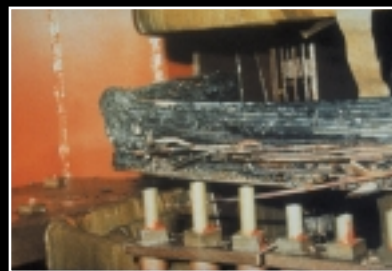
From left to right, the tan-colored paper on the upper winding is intact but burned out below. Next, paper is completely burned out to the right but not left. Last, copper strands have melted.
