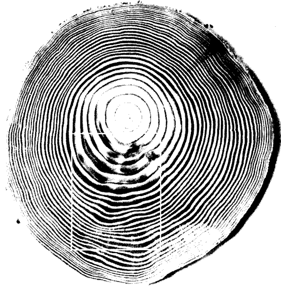
Figure 12.—Stem cross section of softwood with compression wood where the growth rings are wider and darker, within the rectangle.
