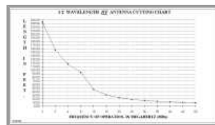
CLICK ON the small graphic to view full size. Half-Wave HF Antenna Cutting Chart.
