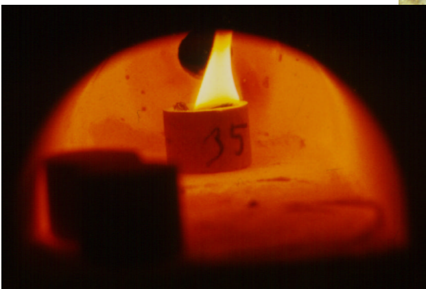
Wood chip in cupel to aid melting
