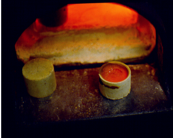
A cupel just out of the muffle furnace. The staining on the left side of the cupel is adsorbed litharge
